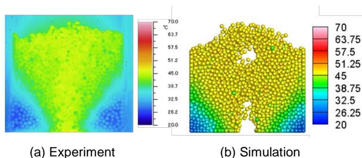
Figure 1 Particle temperature distributions
